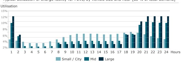
Typical utilization of charge facility for PEVs, by vehicle size and hour [as % of total demand]
